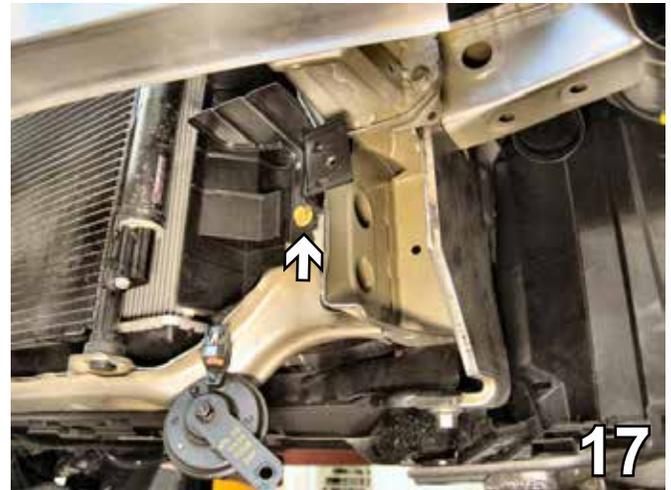
17. Using the 12MM socket, remove the metric bolt from the lower part of the horn shield. Set shield aside. It will not be reinstalled.
