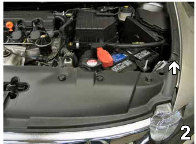
2. To the rear of the driving light, remove a Christmas tree pushpin. Set pushpin aside to be reinstalled later. Do this to both sides of the vehicle.
