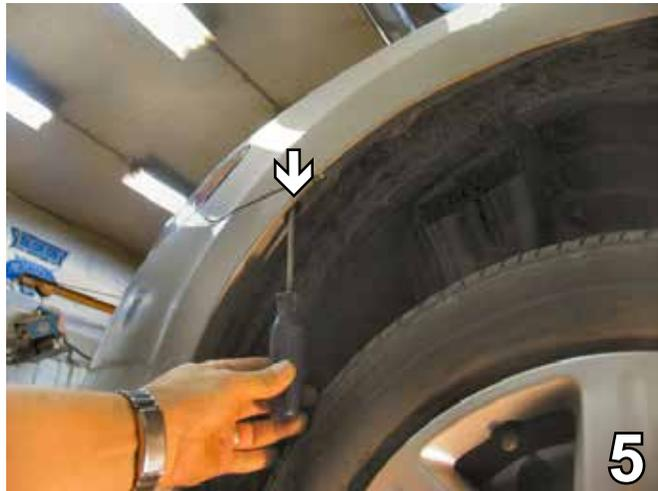
5. Just forward of the front tire, in an opening between the front fascia and the wheel well, use a Phillips screwdriver to remove the screw. Do this to both sides of the vehicle. Set screws aside to be reinstalled later.
