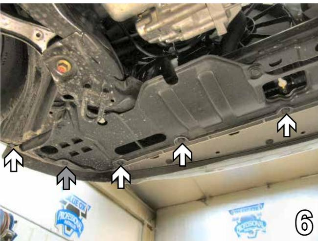
6. Along the bottom edge of the fascia, remove eight push pins, as indicated by the white arrows in the photo above. Do not remove the pushpin found second from either outer edge of the fascia as indicated by the grey arrow in the photo above.
