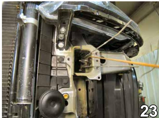
23. Insert 3/8-16 nut plates through the frame rail opening and align with the three drilled holes. Insert 3/8-16 x  $1\frac{1}{2}$ " hex bolts and 3/8" lock washers and tighten. Do this to both sides of the vehicle.
