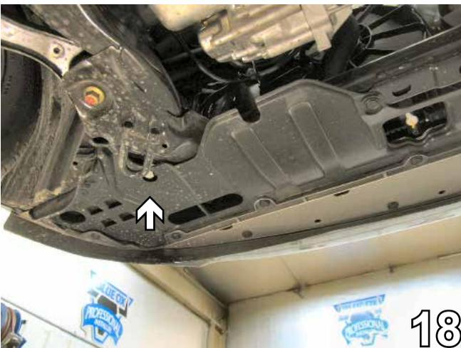
18. Underneath the driver's side, using a 17MM socket, remove the metric bolt from the lower suspension.
