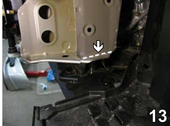
13. Using a reciprocating saw, cut the lip found at the bottom of the radiator support (dotted lines in graphic) to gain access to the area beneath it. Do this to both sides of the vehicle.
