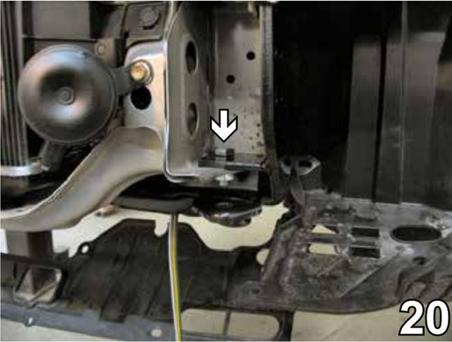
20. Align support plate so  $\frac{1}{2}$ -13 x  $1\frac{1}{4}$ " hex bolt can be inserted into the support plate and through the bottom of the radiator support. Tighten with  $\frac{1}{2}$ " flat washer,  $\frac{1}{2}$ " lock washer, and  $\frac{1}{2}$ -13 hex nut. Finish tightening the metric bolt under the lower suspension.
