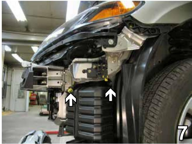
7. On the driver's side, use a 10MM socket to remove two metric bolts securing the air baffle. Pull down to remove. Set bolts and air baffle aside to be reinstalled later.
