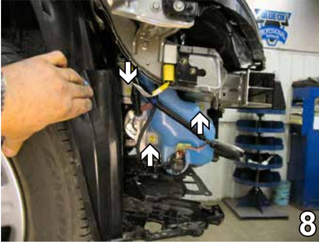
8. On the passenger's side, disconnect and plug the windshield washer reservoir hoses. Disconnect the electrical cable of the windshield washer reservoir pump. Using a 10MM socket, remove three metric bolts from the reservoir. Move the reservoir down and guide the hoses out through the loops found near the top of the windshield washer reservoir. Set bolts and reservoir aside to be reinstalled later.
