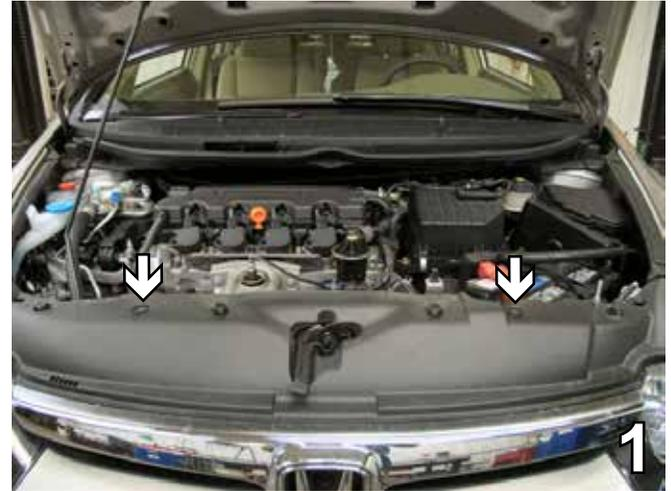
1. Remove two push pins from the top of the fascia. Set push pins aside to be reinstalled later.
