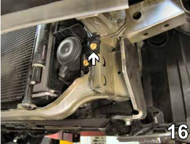
16. Using the 12MM socket, remove the metric bolt from the horn shield on the radiator support on the passenger's side. Hang horn over the lower radiator support ensuring it is out of the way.
