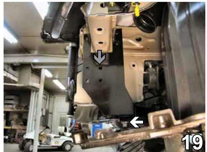
19. On the driver's side, place the support plate against the radiator support and frame. Guide upward until it surrounds the frame side extension. Hold the endplate steady and insert the existing metric bolt, from step 19, underneath the endplate and up into the bolt hole for the lower suspension, as indicated by the white arrow in the photo above. Tighten with the 17MM socket. Do not over tighten as the endplate may need minor adjustments.
