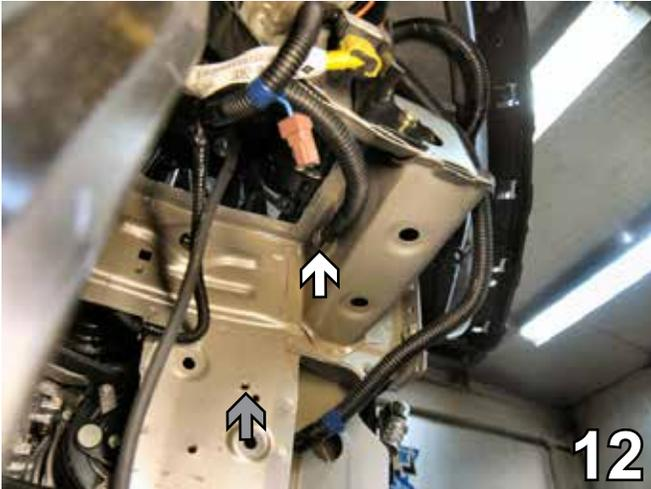
12. On the passenger's side, use a 10MM socket to remove a ground wire from the frame rail. Relocate the ground wire to the rear of the frame extension. The grey arrow is the existing location of the bolt, the white arrow shows where it will be relocated.
