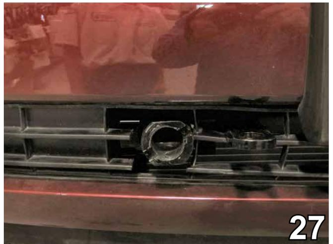
27. Align the fascia to its original position and, using a hack saw blade, trim necessary openings in the grille for the attachment tabs and convenience links.
