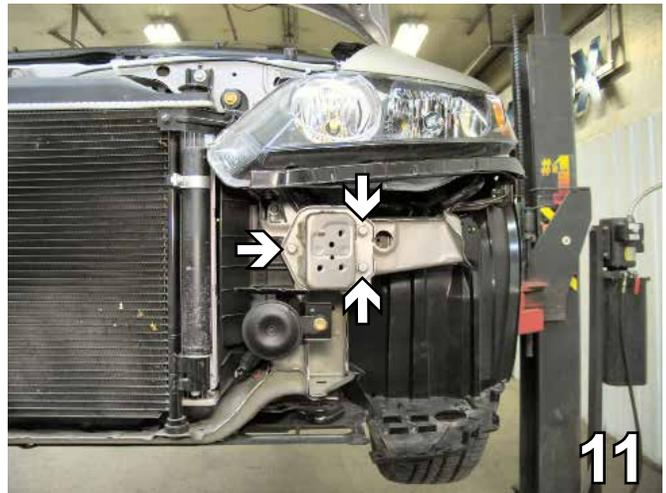
11. Using a 12MM socket, remove three metric bolts from the bumper bracket to gain access to the frame rail. Do this to both sides of the vehicle. Set bolts and brackets aside to be reinstalled later.
