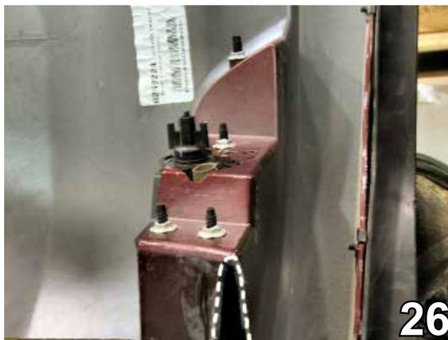
26. On the backside of the fascia, using a utility knife, cut an opening to allow for the fog lights when reinstalling the front fascia. Make a vertical cut of one inch. Make two horizontal cuts (shown) of approximately two inches. Do this to both ends of the fascia.
